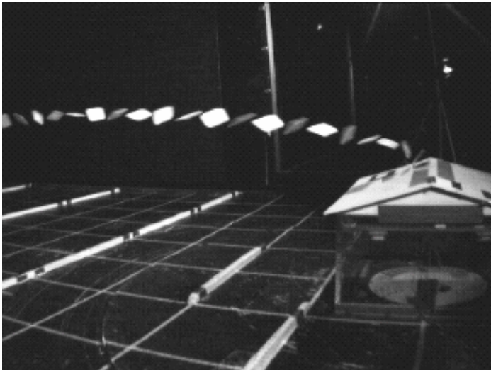
(Left) Flight of a roof sheathing panel from a gable roof in a wind tunnel study simulating Hurricane Andrew conditions. Wind is from right to left, with the (Right) distribution of failure wind speeds as measured over many repeated tests.
